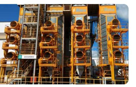
MEGA/TMSA dryers are capable of drying the most diverse types of grains, seeds or not, including soy, corn, rice, beans, sunflower, sorghum, wheat, peanuts, cocoa, among others. In addition, it is a modular technology, which allows the expansion of capacity without the need for modifications to the foundations. Thanks to this differential, the customer can expand the capacity of the dryers in an agile and competitive way.
